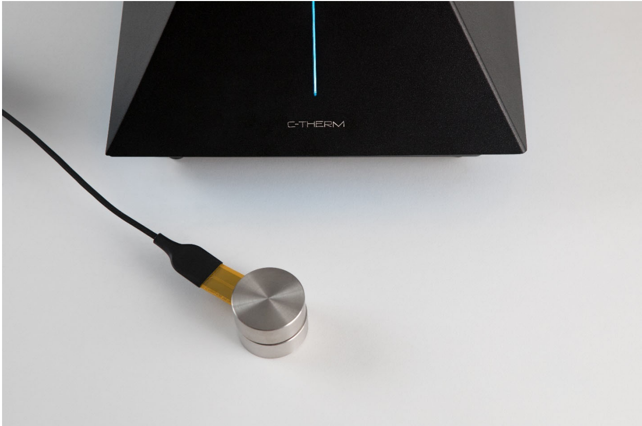
FLEX TPS Sensor sandwiched between stainless steel reference materials.
