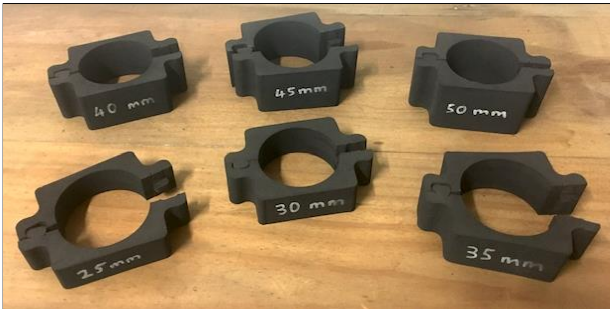
Figure 8. 'Jigsaw' insulation at 5 mm thickness intervals from 25 mm to 50 mm. Note that the 'cropped' teeth always go to the rear of the thermal stack to fit around the sensor wires.
